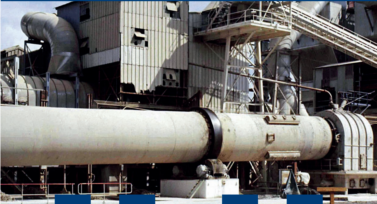
Figure 8: The rear of Southam Kiln 7, commissioned in 1961. Typical post-war welded construction
