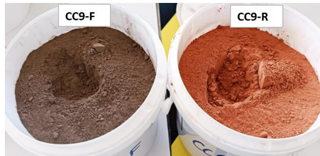
Figure 16: CC9 calcined in flash (left) and rotary kiln (right)
