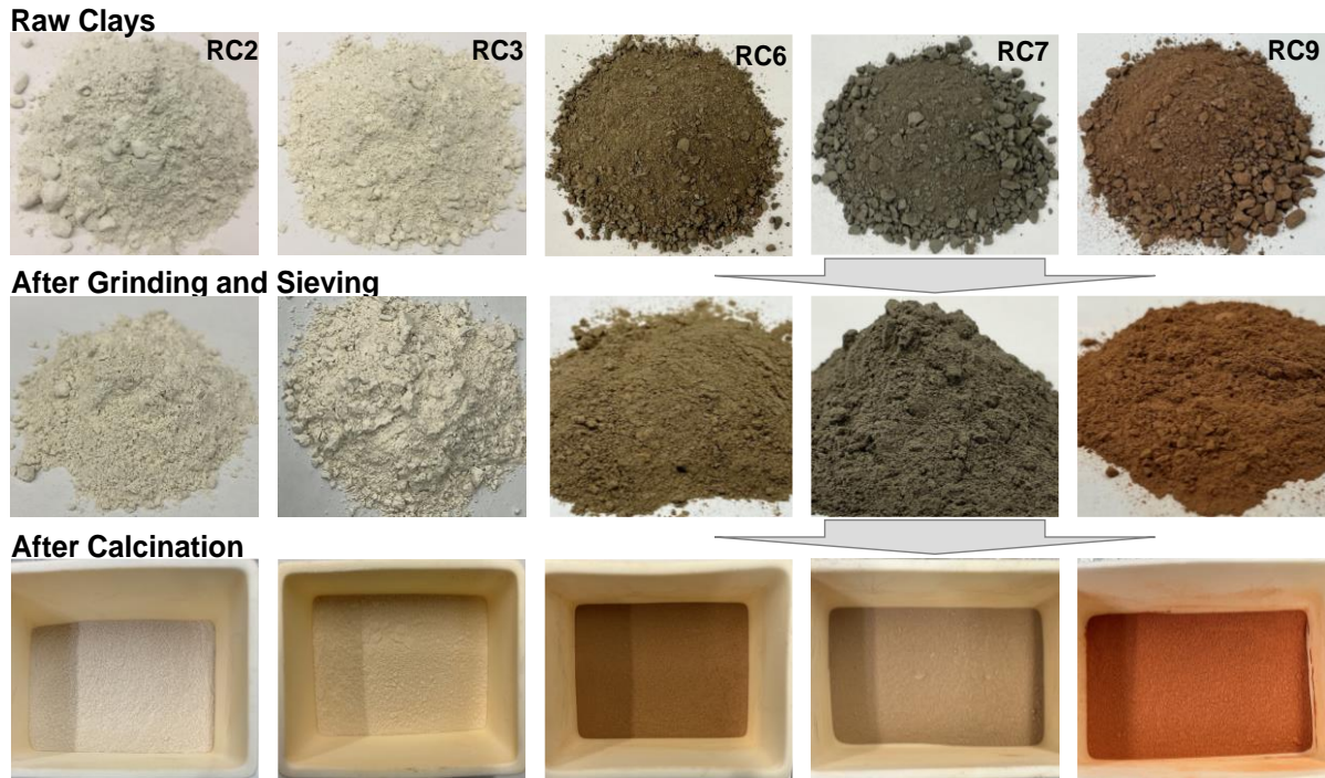
Figure 5: Visual comparison of colour and particle size of the raw clays, ground clays and calcined clays
