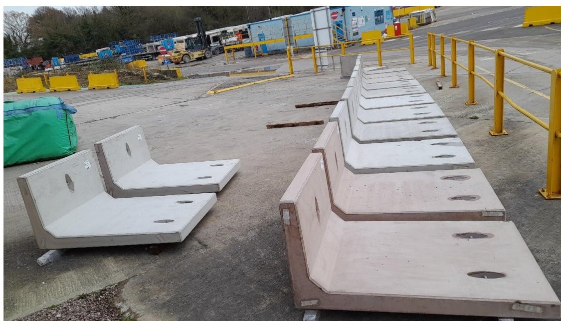
Figure 41: L-shaped retaining wall units produced as part of the Re-C3 project using the different calcined clays
