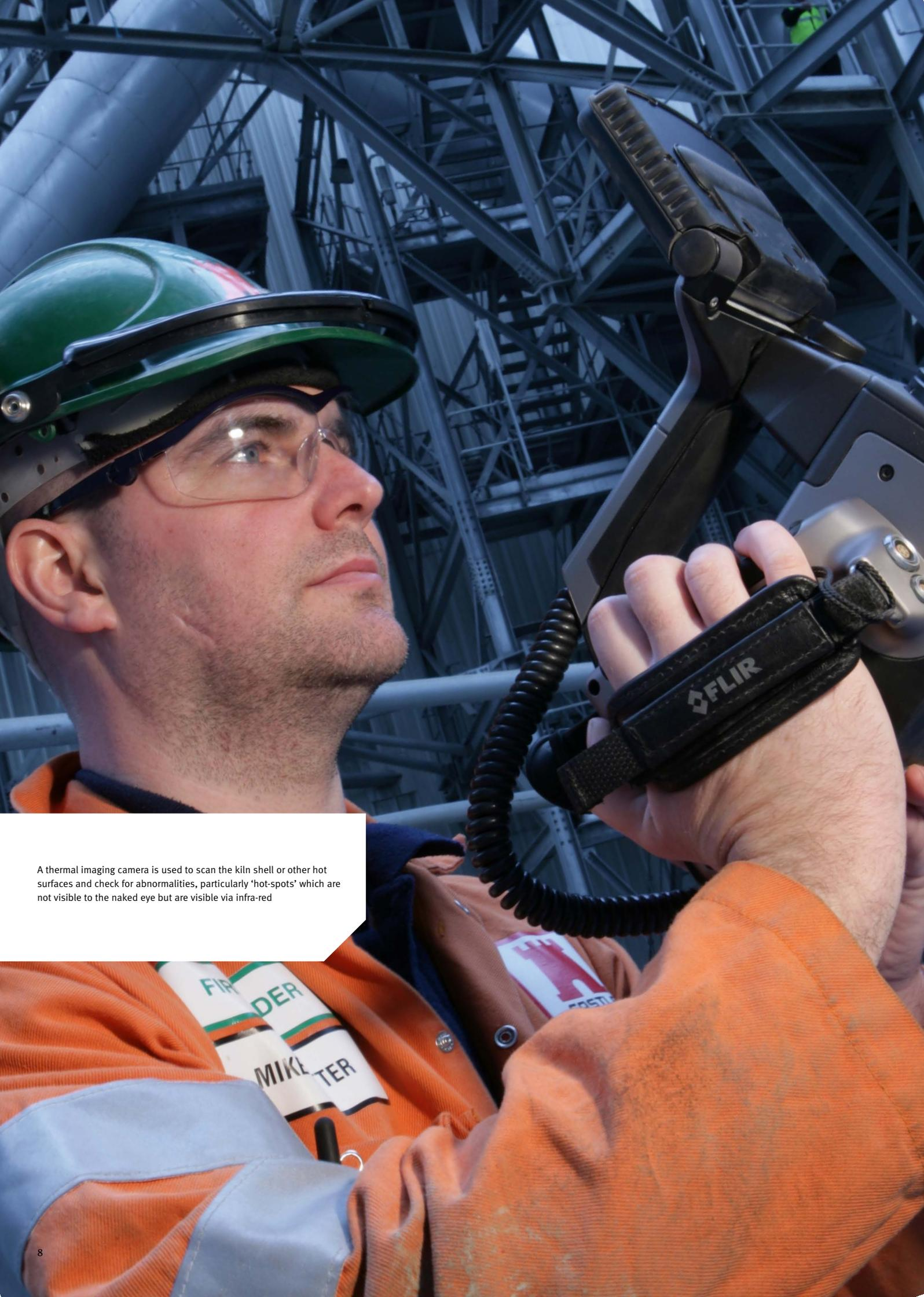
A thermal imaging camera is used to scan the kiln shell or other hot surfaces and check for abnormalities, particularly 'hot-spots' which are not visible to the naked eye but are visible via infra-red
