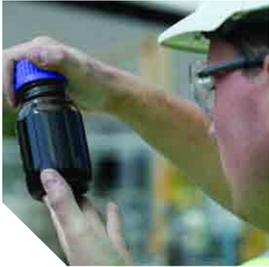
Visual scrutiny of a secondary liquid fuel sample at CEMEX UK
