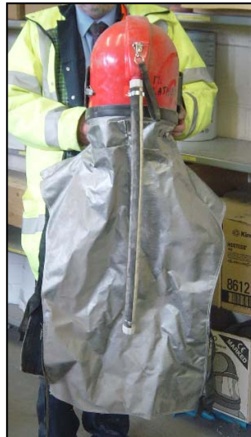
An airflow helmet with combined front and back apron. During operation the helmet is attached to an airline which feeds a constant flow of filtered fresh air from a special low pressure compressor.
