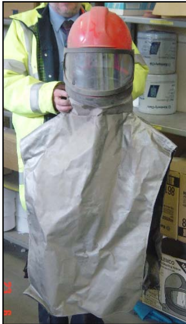
An airflow helmet with combined front and back apron. During operation the helmet is attached to an airline which feeds a constant flow of filtered fresh air from a special low pressure compressor.
