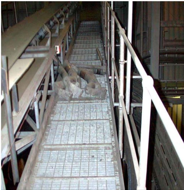
Old pipe sections/fittings left blocking walkway. Similar junk left behind after maintenance work was completed, caused an accident for a contractor.
